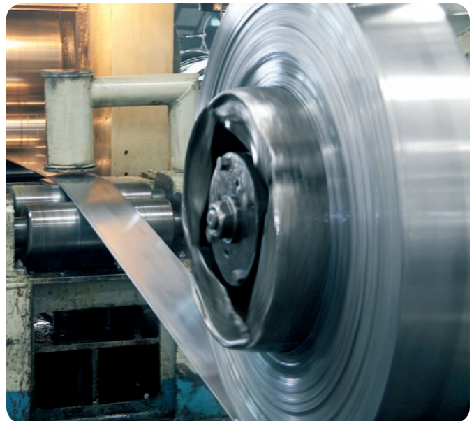
Continuous rolling machine to achieve uniform thickness of plate material
